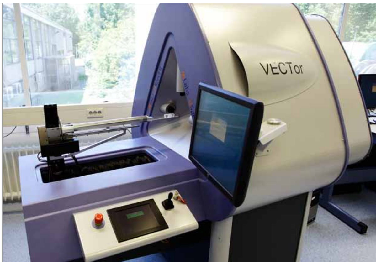
The vector prototype combines three techniques: PET Spect en CT.
